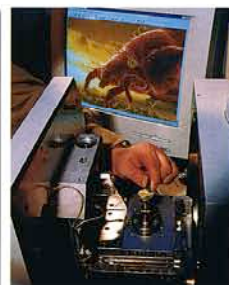
A mite sample is inserted into the chamber of the environmental scanning electron microscope
